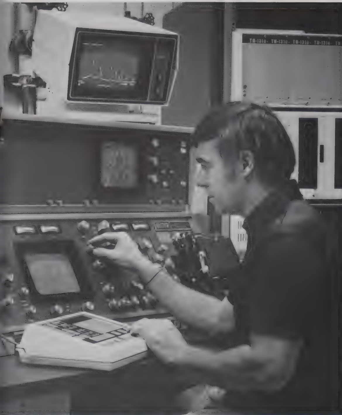
Bob Woods at the controls of his scanning electron microscope. The "tower" at the left is the vacuum chamber into which all specimens are placed for viewing.
